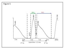
5. Preparative separation of guaiphenesin enantiomers by mixed stream injection. Sample 150 g/l, injection volume 2.7 ml. Column: CHIRALCEL OD 20 $\mu$ m, 250 x 21.2 mm. Mobile phase 20% ethanol in CO<sub>2</sub> at 180 g/min flow rate, 0°C, back pressure 150 bar.
