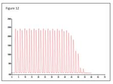
12. Stacked injection separation of warfarin enantiomers. 760 mg warfarin coated on 2 g Daiso C-1 (50  $\mu$ m) packed into an extractor (100 x 10 mm) with 30 second injection time. Conditions as for Figure 11. Separation time 6.3 minutes, cycle time 3.5 minutes.
