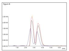
8. Chromatograms of benzoin enantiomers. Blue line: 36 mg (3 ml @ 12g/l) in methanol; black line: 48 mg extraction injection, red line: 62 mg extraction injection. Extractor operated at 40°C. Column: CHIRALCEL OD 20  $\mu$ m, 250 x 21.2 mm. Mobile phase 3% ethanol in CO<sub>2</sub> at 100 g/min flow rate, 25°C, back pressure 110 bar.
