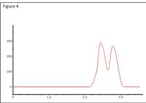
4. Analytical separation of trans-stilbene oxide (TSO) enantiomers by mixed stream and modifier stream injections. Sample TSO, 5 g/l, injection volume 2 ml. Column: CHIRALPAK IA 250 x 21.2 mm. Mobile phase 15% methanol in  $CO_2$  at 100 ml/min flow rate, 40°C, back pressure 100 bar.
