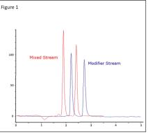
1. Analytical separation of trans-stilbene oxide (TSO) enantiomers by mixed stream and modifier stream injections. Sample TSO, 1 g/l, injection volume 100  $\mu$ l. Column: CHIRALCEL OD-H 150 x 21.2 mm. Mobile phase 15% methanol in CO<sub>2</sub> at 60 ml/min flow rate, 40°C, back pressure 100 bar.
