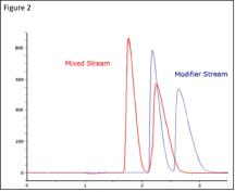
2. Preparative separation of guaiphenesin enantiomers by mixed stream and modifier stream injections. Sample 100 g/l, injection volume 390 µl. Conditions as Figure 1.
