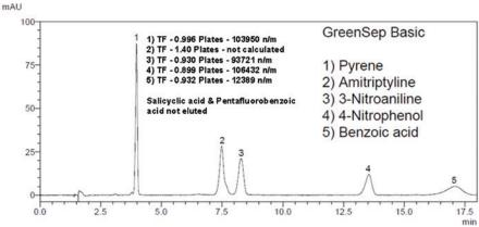
Figure 2: SFC Test Mixture Chromatographed on GreenSep<sup>™</sup> Basic. Operating conditions: column dimensions:  $250 \times 4.6$ mmID, 5um particles, Total Flow: 3 mL/min, Mobile Phase: 0.3 mL/min methanol and 2.7 mL/min CO $_{2^l}$  Back pressure: 150 bar, Column Temperature:  $40^{\circ}$ C, Detection: UV@254nm
