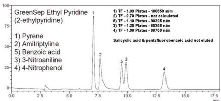
Figure 3: SFC Test Mixture Chromatographed on GreenSep<sup>TM</sup> Ethyl Pyridine. Operating conditions: column dimensions: 250 x 4.6mmlD, 5um particles, Total Flow: 3 mL/min, Mobile Phase: 0.3 mL/min methanol and 2.7 mL/min  $CO_2$ , Back pressure: 150 bar, Column Temperature: 40°C, Detection: UV@254nm
