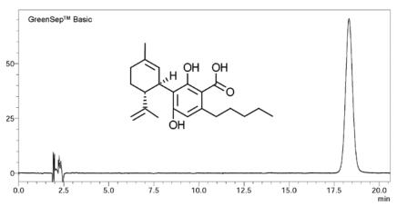
Figure 4: Cannabidiolic acid (CBDA) Chromatographed on GreenSep™ Basic. Operating conditions: column dimensions: 250 x 4.6mmlD, 5um particles, Total Flow: 3 mL/min, Mobile Phase: 0.3 mL/min methanol and 2.7 mL/min CO₂, Back pressure: 150 bar, Column Temperature: 40 C, Detection: UV@254nm
