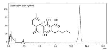
Figure 5: Cannabidiolic acid (CBDA) Chromatographed on GreenSep<sup>™</sup> Ethyl pyridine. Operating conditions: column dimensions: 250 x 4.6mmlD, 5um particles, Total Flow: 3 mL/min, Mobile Phase: 0.3 mL/min methanol and 2.7 mL/min CO<sub>2</sub>, Back pressure: 150 bar, Column Temperature: 40°C, Detection: UV@254nm
