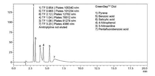
Figure 6: SFC Test Mixture Chromatographed on GreenSep<sup>TM</sup> Diol. Operating conditions: column dimensions: 250 x 4.6mmlD, 5um particles, Total Flow: 3 mL/min, Mobile Phase: 0.3 mL/min methanol and 2.7 mL/min  $CO_{2^{\prime}}$  Back pressure: 150 bar, Column Temperature: 40°C, Detection: UV@254nm
