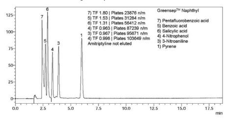
Figure 7: SFC Test Mixture Chromatographed on GreenSep<sup>TM</sup> Naphthyl. Operating conditions: column dimensions: 250 x 4.6mmlD, 5um particles, Total Flow: 3 mL/min, Mobile Phase: 0.3 mL/min methanol and 2.7 mL/min  $CO_2$ , Back pressure: 150 bar, Column Temperature: 40°C, Detection: UV@254nm
