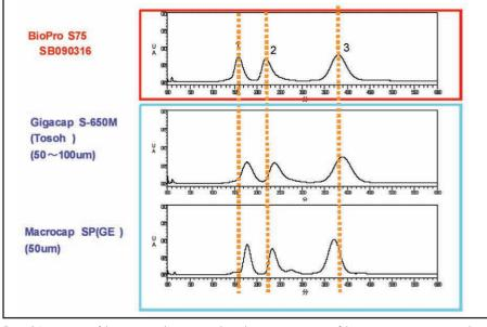
Figure 2 A comparison of three cation exchange materials used to separate a mixture of three proteins using a generic salt gradient. (1) ribonuclease A (MW: 13,700) (2) cytochrome C (MW: 12,400) (3) lysozyme (MW: 14,300)
