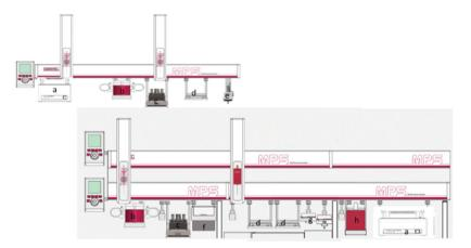
Figure 1: Comparison of Gerstel Multi-Purpose Sampler (MPS) for liquid-liquid extraction and a more complex dual rail system (a:CF200 centrifuge, b:mVap, c:Mvorx, d:sample tray, e:solvent filing station, f:cooled sample tray, g: wash station, h: agitator)
