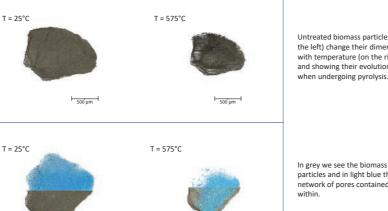
Untreated biomass particles (on the left) change their dimensi with temperature (on the right)
