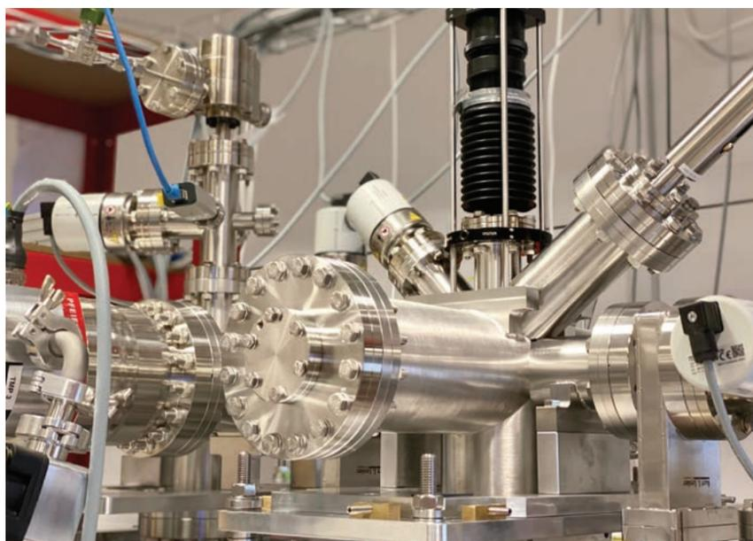
The non-interceptive gas jet beam profiler is flexible and scalable, enabling its use across a range of accelerators, and is not restricted to high-energy storage rings such as the HL-LHC. It can measure the detailed properties of essentially any beam of charged particles in just a few seconds.
