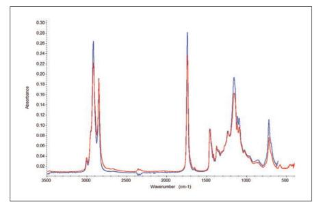
Figure 2. Spectra of oil collected using the AutoATR (red) and a single reflection diamond ATR (blue).
