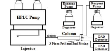
to 50:50. Figure 1b illustrates the phenol detection instrumental set up.
