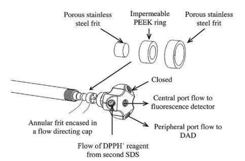
as instrumental setup [11,12,16], such as in the case of PCD reagent, fluorescamine, for the analysis of amino acids [11]. The use of a RF column reduced the number of pumps, coils and mixing devices that are otherwise required in conventional HPLC-PCD analyses using fluorescamine [11]. Ultimately, the RF column enables the complete removal of post column reaction coils, providing high efficiency separation with specific detection.
