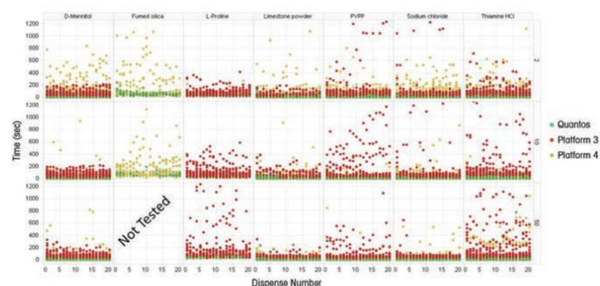
Figure 2: Dispense time (in seconds) for the seven different powder types at 2 mg, 10 mg and 50 mg target doses, measured for three of the platforms tested. Quantos data is shown in green.
