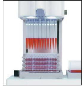
Figure 3. Repeat Dispensing allows quick filling of multiple plates.
