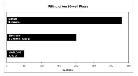
Figure 1. Filling of ten 96-well microplates with 150µl buffer per well is a typical but time consuming procedure using a multichannel pipette. An electronic 96-channel pipette using repeat dispense mode, allows users to perform this task in less than 50 seconds, which is 75% faster than the electronic multichannel pipette.
