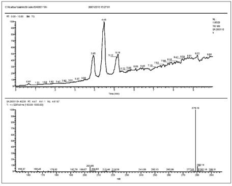
Figure 6. LC-MS analysis of three sulphonamides; MS spectrum shows the predominant MH+ from peak 2 at 4.49 minutes.
