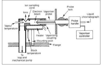
Figure 4. Thermospray source design; Vestal et. al. [11]
