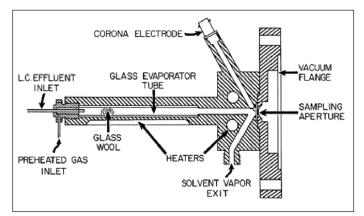
Figure 2. Schematic Diagram of a Corona Discharge Source - Horning et. al. 1975 [6]
