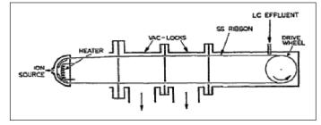
Figure 3. Moving Belt Interface McFadden et. al. 1976 [7]
