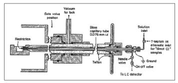
Figure 1. Direct Liquid Introduction Probe - McLafferty et. al. 1973 [2]
