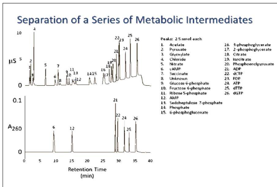
Figure 3. Separation of metabolites on an anion exchange system with a hydroxide gradient.
