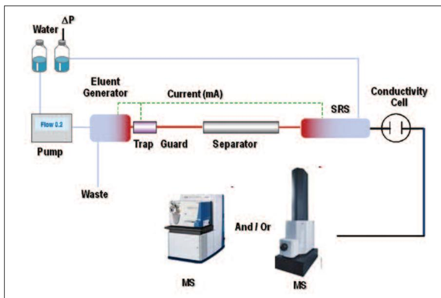
Figure 2. Schematic of a modern IC-MS system.
