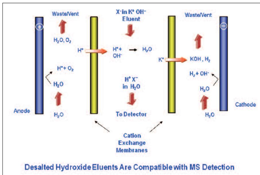
Fig 1 Conversion of a KOH eluent to water using a modern electrolytic anion suppressor
