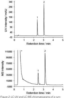
Figure 2: LC-UV and LC-MS chromatograms of a rumwatermelon alcopop sample separated on Chromolith® FastGradient® RP-18 endcapped 50-2mm analytical monolithic silica column. Top: UV, 500nm; bottom: neg. ESI-MS (m/z 140 – 850), base peak chromatogram (BPC). Mobile phase A: acetonitrile, mobile phase B: 20 mM ammonium acetate pH 4.70; gradient: 0' 100% B, 0.5' 100% B, 4.5' 50% B, 5.5' 50% B. 1: Amaranth, 2: Allura Red AC. Asterisk: matrix components (saccharose, citric acid).
