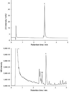
Figure 4: LC-UV and LC-MS chromatograms of an aperitif sample separated on Chromolith® FastGradient® RP-18 endcapped 50 x 2mm analytical monolithic silica column. Top: UV, 500 nm; bottom: neg. ESI-MS (m/z 100 – 850), BPC. Mobile phase A: acetonitrile, mobile phase B: 20mM ammonium acetate pH 4.70; gradient: 0' 100% B, 0.5' 100% B, 4.5' 50% B, 6.5' 50% B. 1: Sunset Yellow FCF, Q: quinine. Asterisk: matrix component (saccharose) eluting in void volume.
