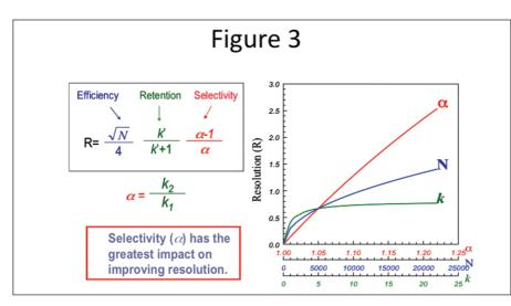
Figure 3. Selectivity ( $\alpha$ ) is a function of resolution, particle size (dp) and retention factor (k').
