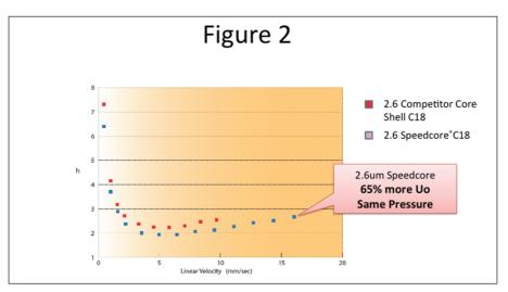
Figure 2. Van-Deemter curve for 2 core-shell, highlights how 65% greater linear velocity (Uo)can be achieved for the same backpressure, giving a greater usable flow rate range.
