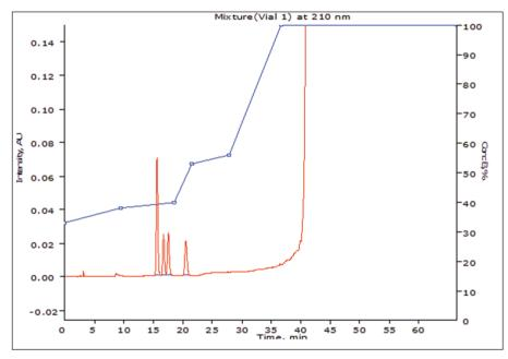
Figure 1. Separation of four isomers that ChromSwordAuto optimised automatically with Agilent 1200 LC system. The resolution (Rs) is 2.2, 1.6 and 4.6 for three peak pairs correspondently
