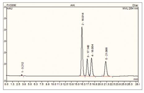
Figure 2. Reproducing a method optimised automatically with Agilent 1100 instrument with Agilent 1100 system. Rs is 2.2, 1.7 and 4.6 for three peak pairs correspondently
