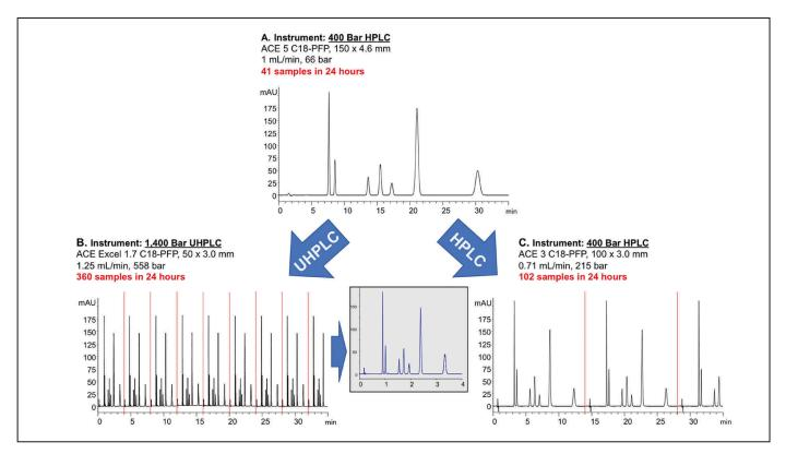
Figure 1: Increasing sample throughput of an existing isocratic HPLC method (A) using UHPLC (B) and modified HPLC (C) options. Mobile phase: MeCN:H<sub>2</sub>O (3:7 v/v), Injection volume: (A) 5 µL, (B) 0.7 µL, (C) 1.4 µL, Detection: UV (214 nm), Sample: 1. 1,2,3-Trimethoxybenzene, 2. 1,2,4-Trimethoxybenzene, 3. 1,4-Dimethoxybenzene, 4. Methoxybenzene, 5. 1,3-Dimethoxybenzene, 6. 1,3,5-Trimethoxybenzene, 7. Toluene.
