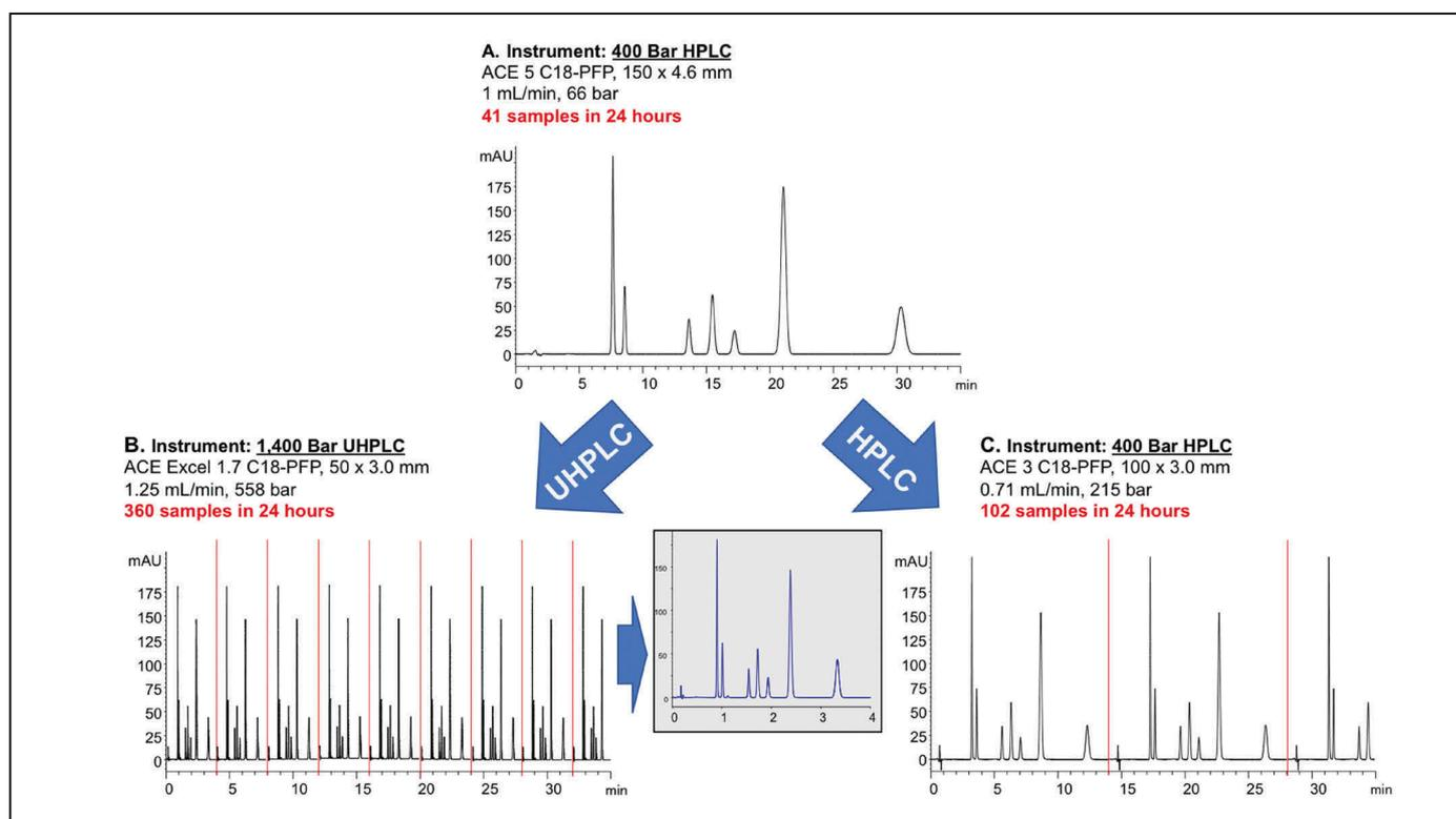
Figure 1: Increasing sample throughput of an existing isocratic HPLC method (A) using UHPLC (B) and modified HPLC (C) options. Mobile phase: MeCN:H<sub>2</sub>O (3:7 v/v), Injection volume: (A) 5  $\mu$ L, (B) 0.7  $\mu$ L, (C) 1.4  $\mu$ L, Detection: UV (214 nm), Sample: 1. 1,2,3-Trimethoxybenzene, 2. 1,2,4-Trimethoxybenzene, 3. 1,4-Dimethoxybenzene, 4. Methoxybenzene, 5. 1,3-Dimethoxybenzene, 6. 1,3,5-Trimethoxybenzene, 7. Toluene.
