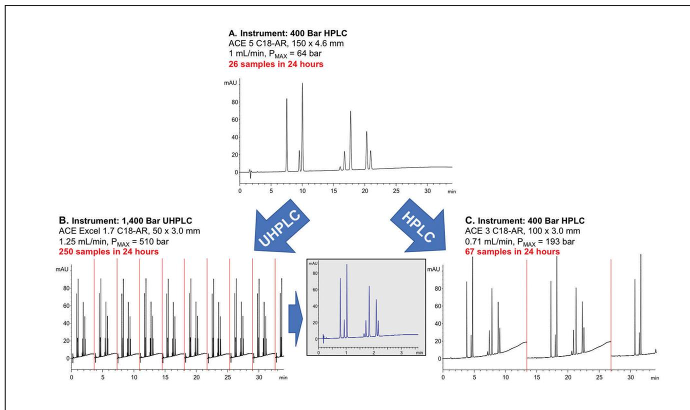
Figure 2: Increasing sample throughput of an existing gradient HPLC method (A) using UHPLC (B) and modified rapid HPLC (C) options.
