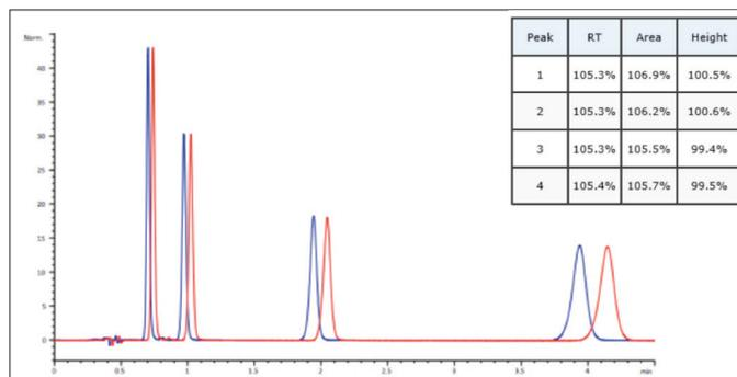
Flow rate reduced by 5%. Retention and peak area change – peak height ratio (PHR) remains constant.
