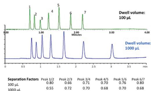
Figure 1 demonstrates the effect with the two systems clearly having different retention times for some of the peaks, looking at the earlier eluting compounds the effect is quite dramatic.
