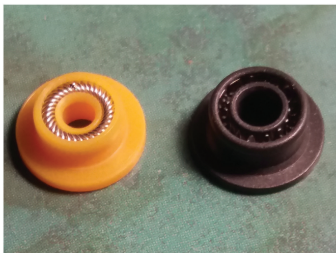
Figure 2: Two common pump seals, a high molecular weight polyethylene for UHPLC and a PTFE filled graphite for lower pressure.
