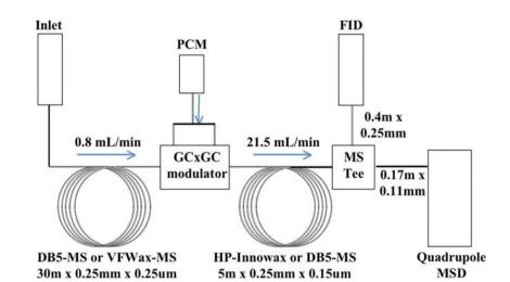
Figure 3: GCxGC-FIDqMSD configuration showing both column sets
