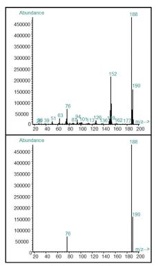
Diagram 7: SIM has less noise and allows more ions of the m/z range through to the MS detector therefore giving higher sensitivity than SCAN window, giving more data points per peak, as more cycles per second and longer dwell times on each ion are enabled.
