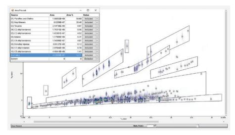
Figure 1. GC×GC–FID colour plot of naphtha, showing the pre-defined stencil regions and integrated peaks (denoted by '×' symbols). This information is translated into an area percent table (inset) that provides a fast overview of sample composition – in this case, >99.9% of the total sample composition is classified using the stencil regions.
