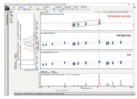
Figure 2. Classification of C<sub>11</sub>-alkylbenzenes in a heavy alkylate using GC×GC with dual FID/TOF MS detection. The excellent retention-time correlation (highlighted in the left-hand panel for the selected peak) allows stencils to be transferred easily from TOF MS to FID.
