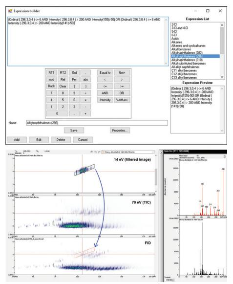
Figure 3. Top: Scripting expression used to classify the  $C_{12}$ -alkylnaphthalenes. Bottom: Use of this expression to filter the 14 eV TOF MS data from the analysis of the heavy alkylate, and generate a stencil for this compound group that can be applied to the FID data.
