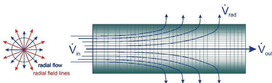
Figure 1: Hollow fibre flow pattern  $V_{rad}$ : radial cross flow;  $V_{in}$ : pump flow;  $V_{out}$ : detector flow
