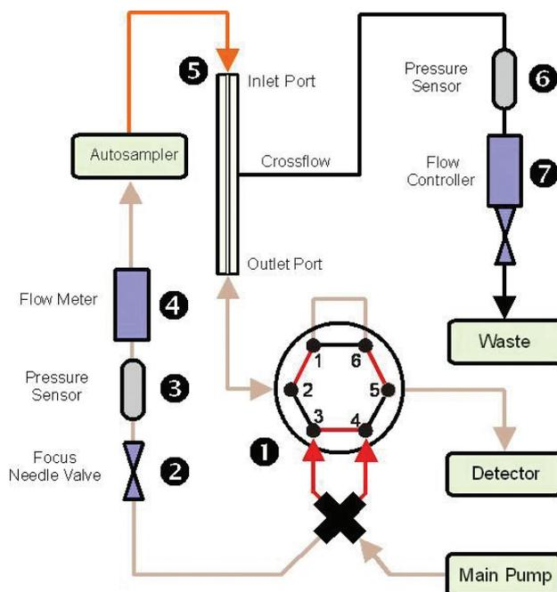
Figure 3: Schematic view of the flow pattern and control elements used in the DUALTEC instrument:
