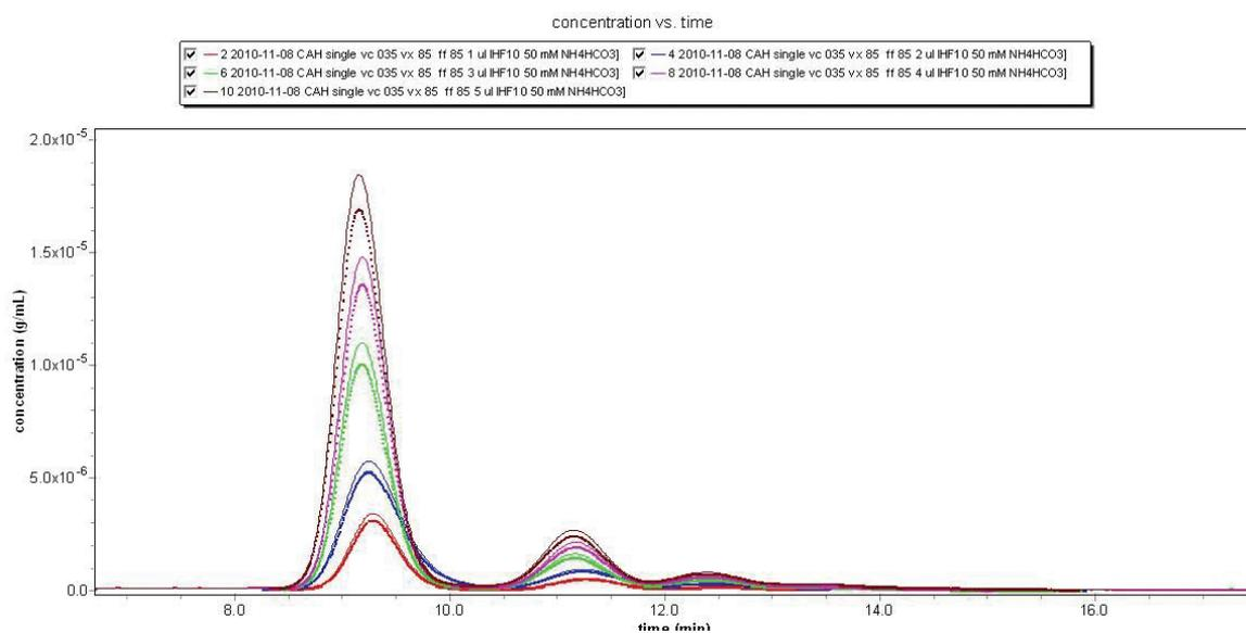
Figure 4: Separation of carbonic anhydrase (1 mg/ml) with hollow fibre (800µm) cartridge, injection amounts increase from 1µg to 5µg, UV signal at 280nm (dotted line: concentrations calculated from UV data)
