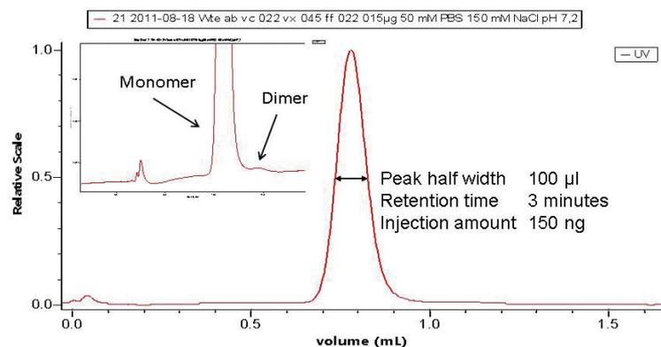
Figure 7: analysis of a monoclonal antibody; UV signal at 210nm
