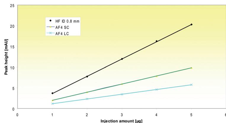
Figure 5: Carbonic anhydrase separation; peak height as a function of injection amount compared to calculated peak heights on AF4 channels SC and LC with 350µm channel height
