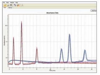
Figure 4. ActiPix D100 traces of 214 nm absorbance at window 2 (red) and window 3 (blue). Overlay of 9 consecutive runs with injection of 34 nL of the sample solution. Run sequence: (i) 20 mbar, 20 kV, 3.5 min; (ii) 0 mbar, 0 kV, 0.5 min; (iii) 50 mbar, 15 min.
