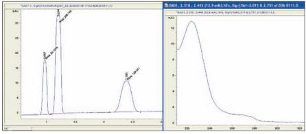
Figure 3. Absorbance at 214 nm from Agilent 7100 detector at the first window; 20 mbar, 20 kV for 3.5 min. Analyte migration order lidocaine, phenylmethanol, benzoate. Inset: UV spectrum for the 3rd peak (benzoate).
