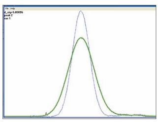
Figure 5. Example of experimental data and fitting for Taylor dispersion analysis. Blue and black lines are absorbance output traces for benzoate from the second and third windows, respectively. The green line the result of convoluting the blue line with a Gaussian function that has a standard deviation of 5.891 s.
