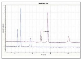
Figure 6. Traces at second and third windows (blue and red, respectively) for 30 mbar, 10 kV; ActiPix D100 detector, 214 nm. Analyte migration order lidocaine, phenylmethanol, benzoate.
