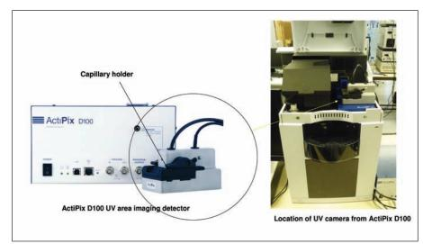
Figure 1. Integration of the ActiPix D100 UV imaging system and the Agilent 7100 CE system.
