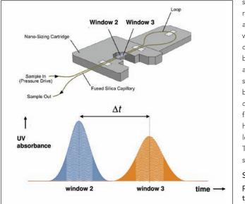
Figure 2. Schematic of ActiPix sizing cartridge and peak broadening in pressure-driven flow between second and third windows.
