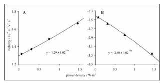
Figure 7. Measured effective mobility of A, lidocaine and B, benzoate with applied voltages of 5, 10, 15 & 20 kV plotted against dissipated power density. The fitted line extrapolated to zero gives the effective mobility at zero power. The fit assumes a mobility increase of 2% / °C and indicates an estimated temperature increase of 10 °C m  $W^1$ .
