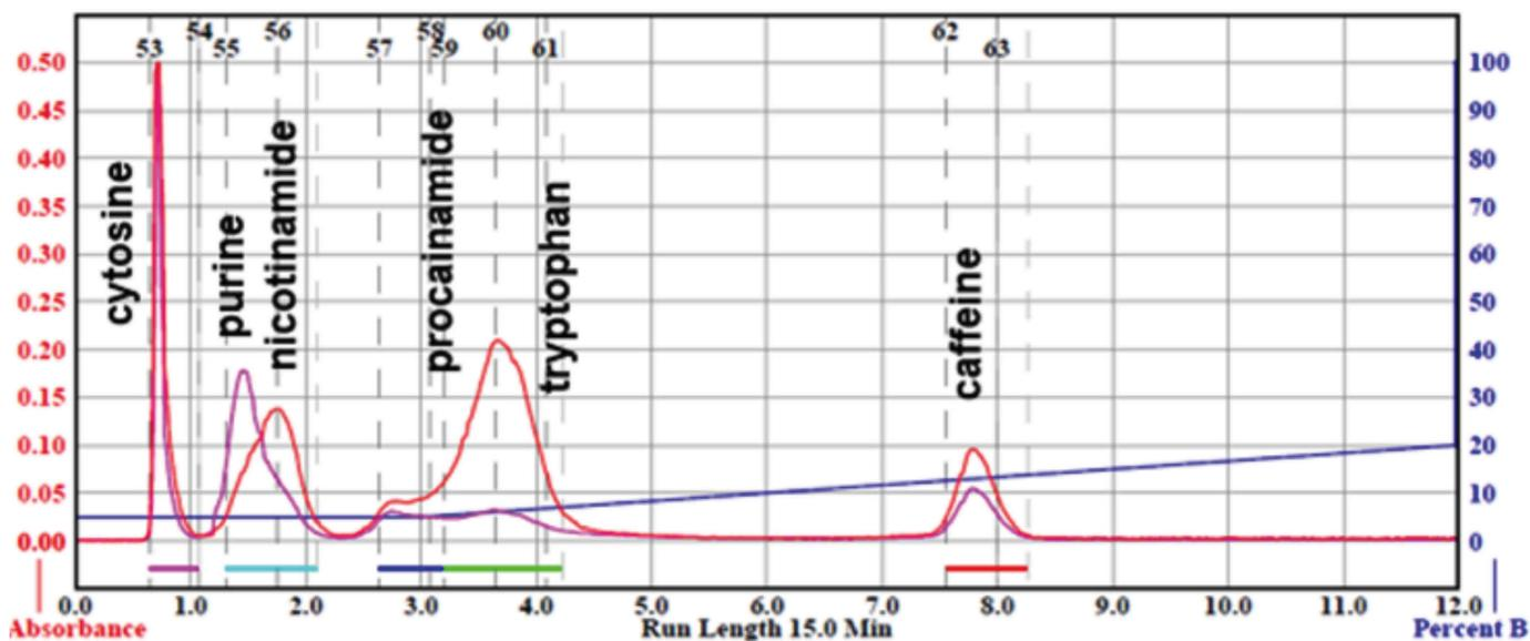
Figure 4. Flash Chromatography Polar Test Mix on 5-20% of B in A for 9 min gradient – Solvent A: Water with 10mM ammonium formate; Solvent B: 95% ACN in water with 10 mM ammonium formate; Teledyne ISCO 15.5g GOLD C18 (20-40 $\mu$ m) Redisep, 30 mlmin<sup>-1</sup>, 220 nm and 254 nm.
