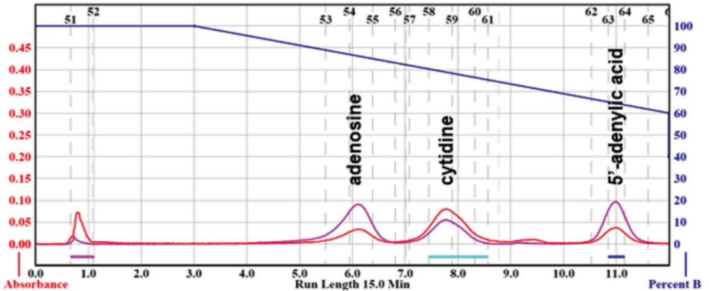
Figure 6. Flash Chromatography Polar Test Mix on 100-60% of B in A for 9 min gradient – Solvent A: Water with 10 mM ammonium formate; Solvent B: 95% ACN in water with 10mM ammonium formate; Teledyne ISCO 12g GOLD Silica (20-40  $\mu$ m) Redisep, 30 mlmin<sup>-1</sup>, 220 nm and 254 nm.
