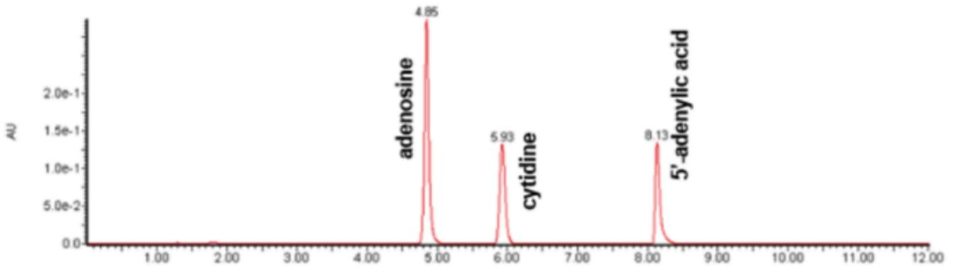
Figure 5. HILIC Analytical on 100-60% of B in A for 6 min gradient – Solvent A: Water with 10 mM ammonium formate; Solvent B: 95% ACN in water with 10mM ammonium formate; Atlantis HILIC Silica column 4.6x100mm, 5 $\mu$ m
