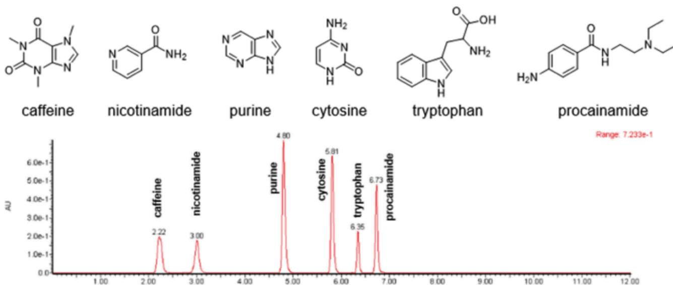
Figure 1. HILIC Analytical Polar Test Mix on 100-60% of B in A for 6 min gradient – Solvent A: water with 10 mM ammonium formate; Solvent B: 95% ACN in water with 10mM ammonium formate; Atlantis HILIC Silica column 4.6x100mm, 5 $\mu$ m.
