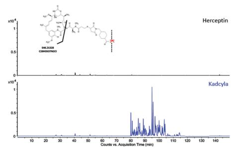
Figure 7: All-ions MS/MS chromatograms of the Herceptin and Kadcyla tryptic digest. The ion at m/z 547.2206 was extracted at high mass accuracy. [1]
