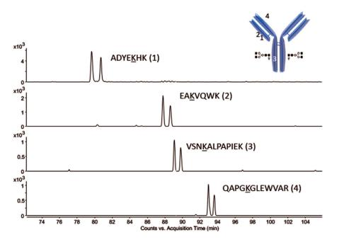
Figure 8: Extracted ion chromatograms of selected peptides showing the appearance of isomeric conjugated peptides. [1]
