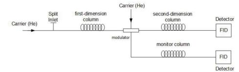
Figure 2. Diagram of the flow modulation setup.
