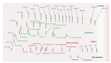
Figure 4. 2D-plot of a gravimetric blend reference sample
