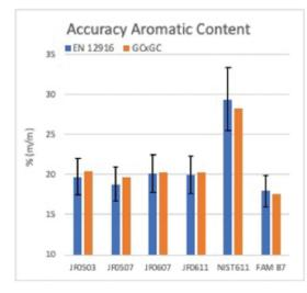
Figure 6. GCxGC aromatic content versus EN 12916:2016 (confidence levels based on Reproducibility calculation EN 12916:2016
