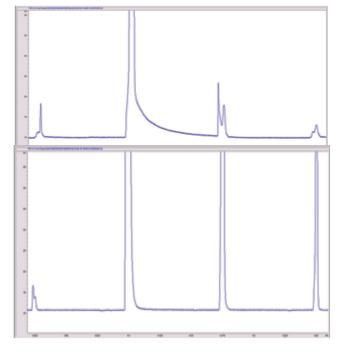
Figure 1. Examples of Standard Flow Modulation (top chromatogram) and AC Flow Modulation (bottom chromatogram of Cyclohexane
