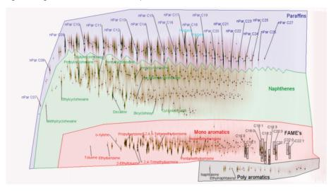
Figure 3. Typical 2D - plot of a Diesel B7
