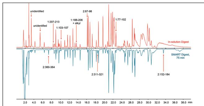
Figure 4. Mirror plot of the TIC chromatogram for the in-solution-digested sample denatured with heat (In-Solution, Heat) and the reduced SMART Digest sample (SMART Digest, 75 min). Peak labels give annotation to light (1) or heavy (2) chains, respectively, and sequence position.
