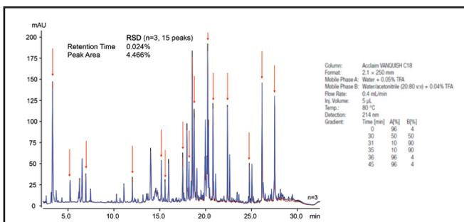
Figure 3. UV chromatogram overlay from three separate SMART digestions from the same mAb, conducted by three individual operators. The 15 marked peptides in each sample were used for inter-user/inter-day RSD value calculations.
