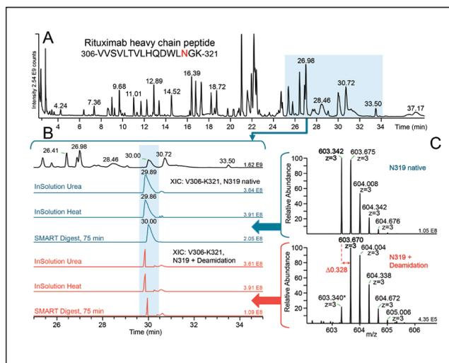
Figure 8. Total ion current chromatogram of the reduced SMART Digest sample, 75 min (A), and extracted ion current chromatograms (B) for the peptide V306-K321 in the native and the deamidated form for the different runs. A comparison of the isotopic distributions of the  $[M+3H]3^+$  ions (C) for the native and deamidated V306-K321 peptide.
