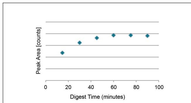
Figure 2. IgG digest profile, monitoring the mAb peptide VSVLTVLHQDWL-NGK for digestion times from 15–90 min using the SMART Digest kit (3).
