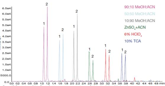
Figure 15: Comparison of the effects of various pretreatment options on Codeine (peak 1) and Hydrocodone (peak 2) Chromatograms are overlaid with time shift to provide clarity [1].
