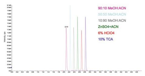
Figure 19: Comparison of the effects of various pretreatment options on MDMA. Chromatograms are overlaid with time shift to provide clarity [1].
