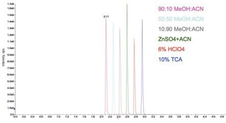
Figure 20: Comparison of the effects of various pretreatment options on Tramadol, Chromatograms are overlaid with time shift to provide clarity [1].
