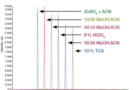
0.0 0.2 0.4 0.6 0.8 1.0 12 1.4 1.6 1.8 20 22 24 26 28 3.0 32 3.4 3.6 3.8 40 42 44 4.6 4.8 min Figure 14: Comparison of the effects of various pretreatment options on amphetamine. Chromatograms are overlaid with time shift to provide clarity [1].
