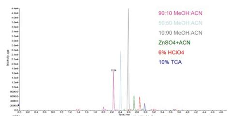
Figure 18: Comparison of the effects of various pretreatment options on EDDP. Chromatograms are overlaid with time shift to provide clarity [1].
