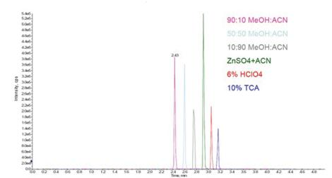
Figure 17: Comparison of the effects of various pretreatment options on Nordiazepam. Chromatograms are overlaid with time shift to provide clarity [1].
