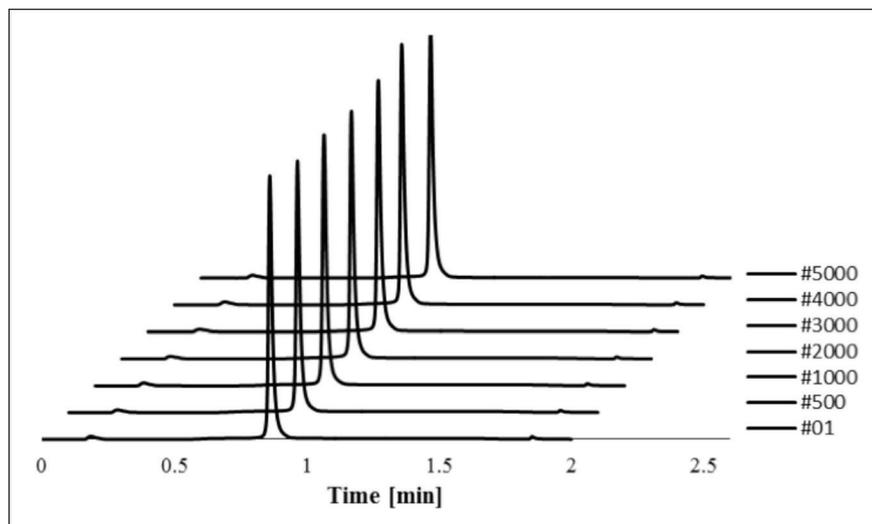
Figure 4: Stability test of immobilised rSPA silica monolith against 10,000 pH shifts using gammarnorm IgG (1 mg/mL) as control for column performance. Chromatographic conditions: Stepwise gradient: 100 mM sodium phosphate pH 7.4/100 mM sodium phosphate pH 2.5; 0.05 min 100/0, 0.05-0.06 min 0/100, 1.10 min 0/100, 1.10-1.15 100/0, 1.15-2.00 min 100/0; flow rate: 2.0 mL/min; detection: 280 nm; injection: 10  $\mu$ L; temperature: 25°C
