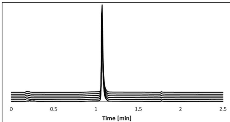
Figure 2: Analysis of 50 injections of cetuximab (1 mg/mL) on immobilised rSPA silica monolith. Only first and every 10th chromatogram is shown. Chromatographic conditions: Stepwise gradient: 100 mM sodium phosphate pH 7.4/100 mM sodium phosphate pH 2.5; 0.25 min 100/0, 0.25-0.26 min 0/100, 1.00 min 0/100, 1.00-1.01 100/0, 1.01-2.50 min 100/0; flow rate: 2.0 mL/min; detection: 280 nm; injection: 10  $\mu$ L; temperature: 25°C
