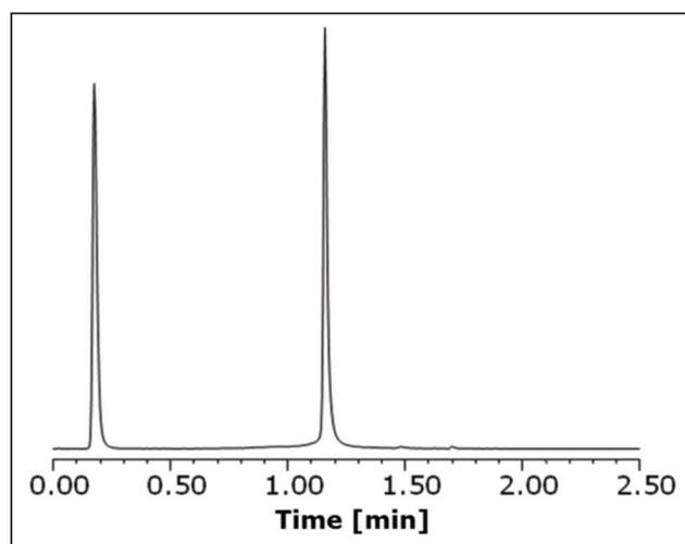
Figure 1: Separation of cetuximab (1 mg/mL) and BSA (1 mg/mL) by immobilised rSPA silica monolith. Chromatographic conditions: Stepwise gradient: 100 mM sodium phosphate pH 7.4/100 mM sodium phosphate pH 2.5; 0.25 min 100/0, 0.25-0.26 min 0/100, 1.00 min 0/100, 1.00-1.01 100/0, 1.01-2.50 min 100/0; flow rate: 2.0 mL/min; detection: 280 nm; injection: 10  $\mu$ L; temperature: 25°C
