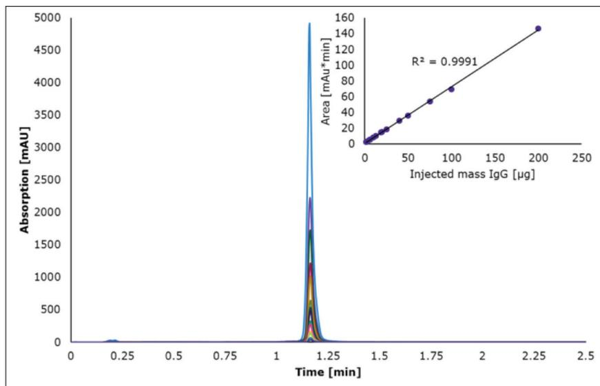
Figure 3: Calibration curve of Cetuximab on rSPA silica monolith ranging from 1.25 µg to 200 µg. Chromatographic conditions: Stepwise gradient: 100 mM sodium phosphate pH 7.4/100 mM sodium phosphate pH 2.5; 0.25 min 100/0, 0.25-0.26 min 0/100, 1.00 min 0/100, 1.00-1.01 100/0, 1.01-2.50 min 100/0; flow rate: 2.0 mL/min; detection: 280 nm; injection: 20 µL; temperature: 25°C
