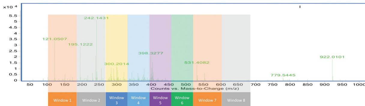
**Fig. 3: Schematics of a wide band quadrupole experiment.** Similar to All Ions, but using the quadrupole to take sequential windows of the mass range to reduce complexity of the MS/MS spectra.
