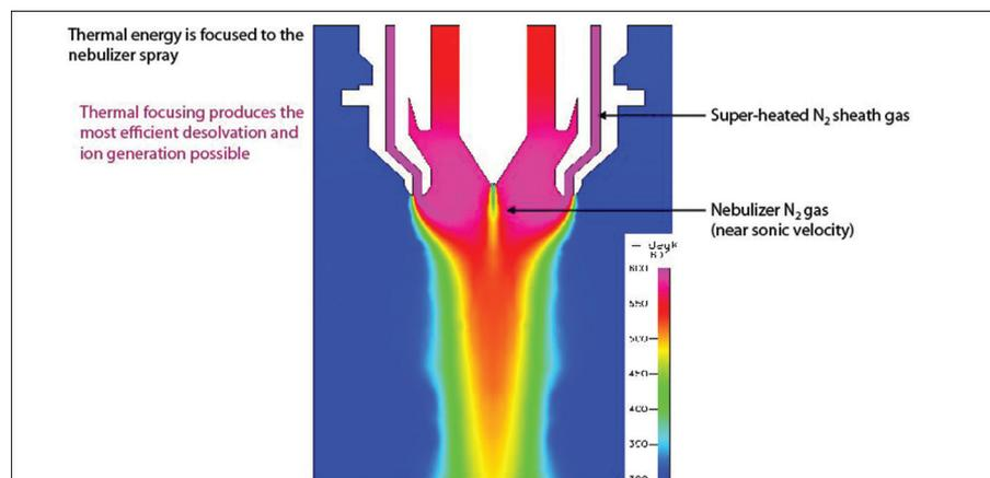
Figure 2. Simulation showing the thermal profile of the Agilent Jet Stream technology. Note the creation of a thermal confinement zone by introduction of a super-heated  $N_2$  sheath gas.
