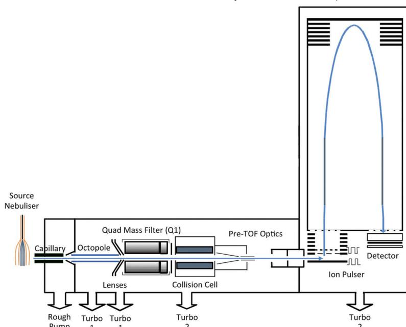
**Fig. 1: Schematics of a TOF instrument.** Basic elements include the source, the quadrupole, collision cell, flight tube and detector.
