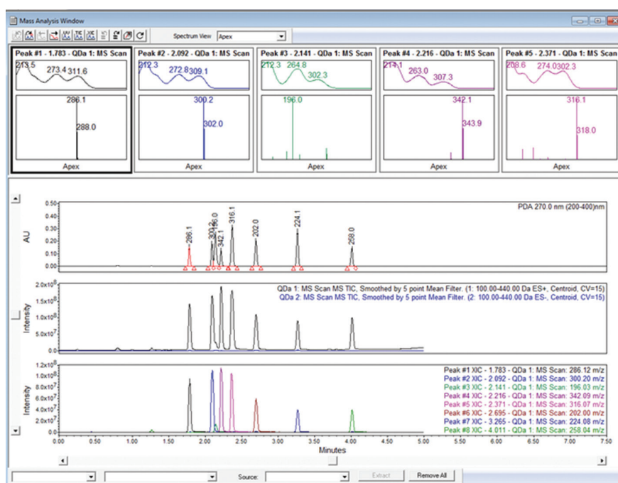
Figure 1. Empower 3 CDS software provides a simple view of mass and UV chromatograms and spectra, enabling fast peak identification and determination of peak homogeneity.
