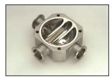
The Robolux Valve makes use of a body (typically machined from 316L stainless steel) which incorporates two traditional weirs located next to each other. On top of this body sits a diaphragm; often manufactured of materials like EPDM, PTFE or silicone the diaphragm is completely moulded and does not have any metal parts. This is an advantage for diaphragm lifecycle.
