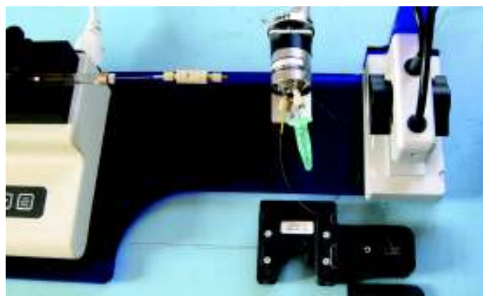
Figure 3: Integrated system for sizing with syringe pump, injection valve and ActiPix detector. Sizing cartridge shown disassembled.
