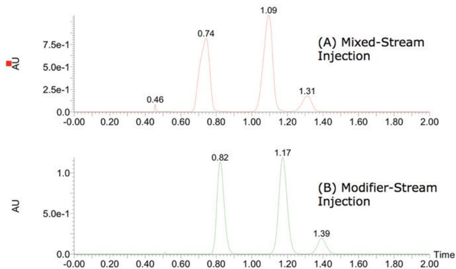
Figure 2: Comparison of UPC<sup>2</sup> chromatograms using mixed-stream and modifier-stream injection techniques.
