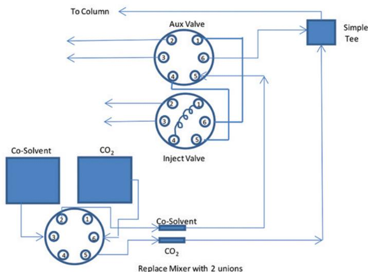
Figure 1: Plumbing diagram for UPC<sup>2</sup> using modifier stream injection.
