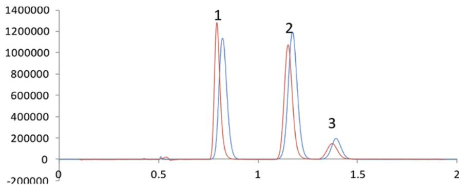
Figure 3: Overlaid chromatograms of the volume-to-volume scaled-up separation on the 19 mm Torus 2-PIC column (red) and on the 3 mm Torus 2-PIC column (blue). Preparative method conditions: 60 mL/min total flow, 15% methanol, 40°C, 124 bar, 200  $\mu$ L injection volume. Analytical method conditions: 1.5 mL/min total flow, 15% methanol, 40°C, 124 bar, 5  $\mu$ L injection volume. Peaks: (1) Caffeine, (2) Theophylline, (3) Theobromine
