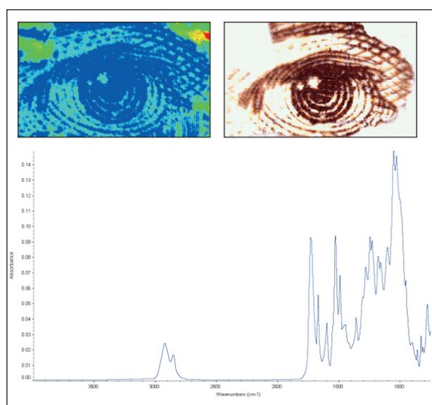
Figure 1. (Upper left) Chemical image of Andrew Jackson's eye on \$20 US currency (Upper right) Video mosaic of Jackson's eye (Lower) Black ink spectrum collected by Tip ATR. Chemical imaging highlights the distribution, while ATR analysis provides detailed spectral information of the ink.
