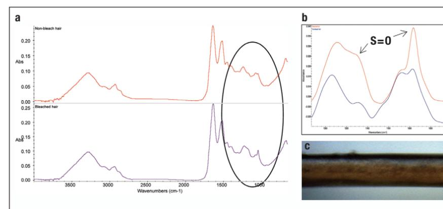
Figure 2. (a) Spectra of non-bleached (red) and bleached (purple) hair. (b) Expanded region showing S=O stretching regions (c) Video image of un-bleached hair fibre.
