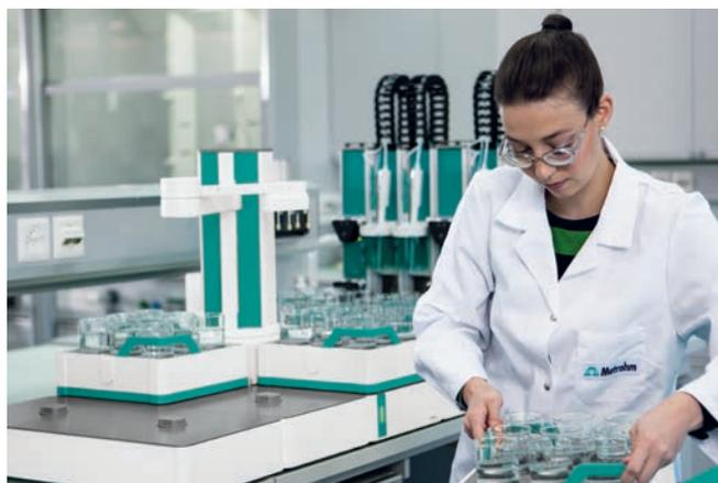
*The OMNIS Sample Robot accommodates up to 175 samples and enables the exchange of racks with already analysed samples while the system keeps analysing.*
