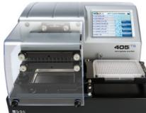
**BioTek** has been awarded US Patent 8,858,718, covering the use of ultrasonic devices to check for clogged manifold tubes and to clean the manifold tubes of a microplate washer automatically. The two features are known as Verify<sup>™</sup> and Ultrasonic Advantage<sup>™</sup> and are available in BioTek's 405 family of microplate washers.
