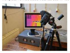
Monitoring a battery cell for hot spots.
