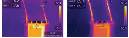
Cables with a low current rating are put to the test. If approved for use, these cables will contribute to keeping the weight of the car low.
