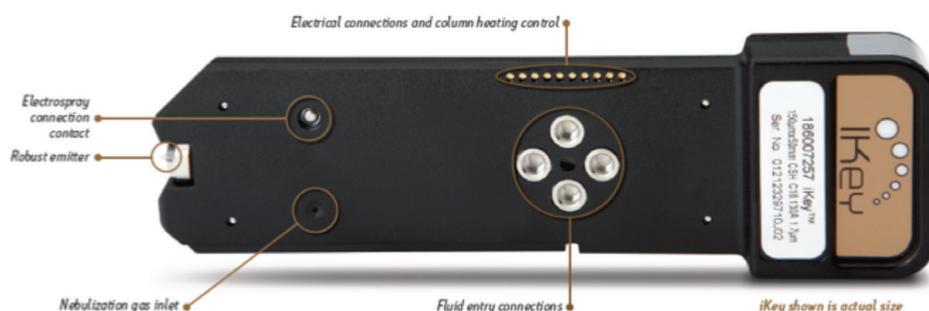
Figure 1. iKey Separation Device
