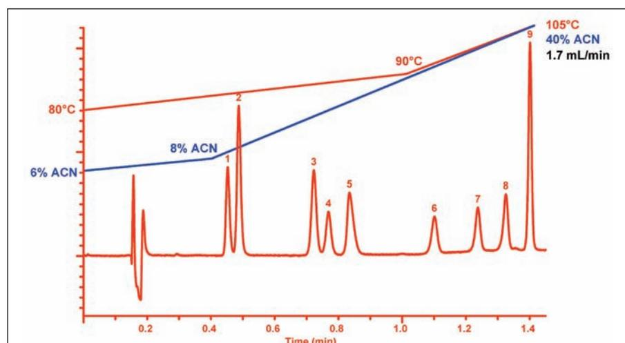
Figure 2. Chromatogram of the separation of a sulfonamide mixture and trimethoprim using a simultaneous solvent and temperature gradient on a Zorbax StableBond C-18 column. For experimental information, see reference [11].
