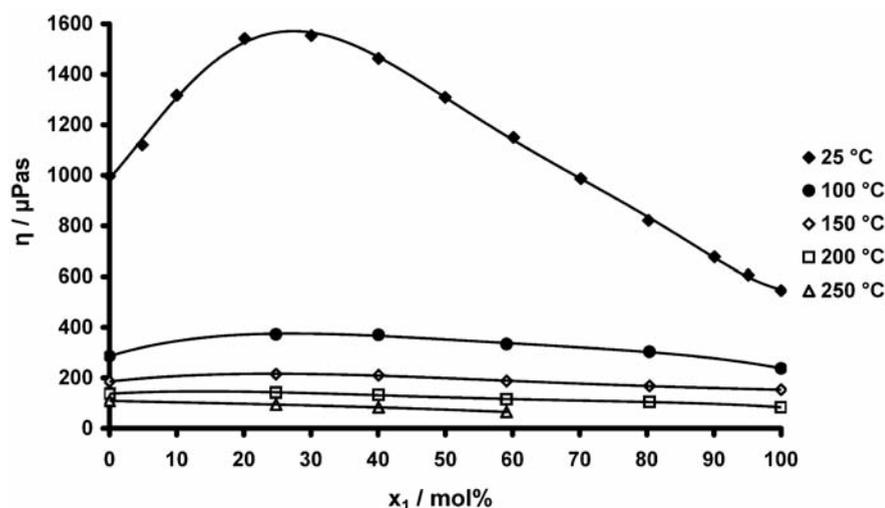
Figure 1. Viscosities of the binary mixture methanol (1) – water (2) at different temperatures. Additional data can be found in reference [15].
