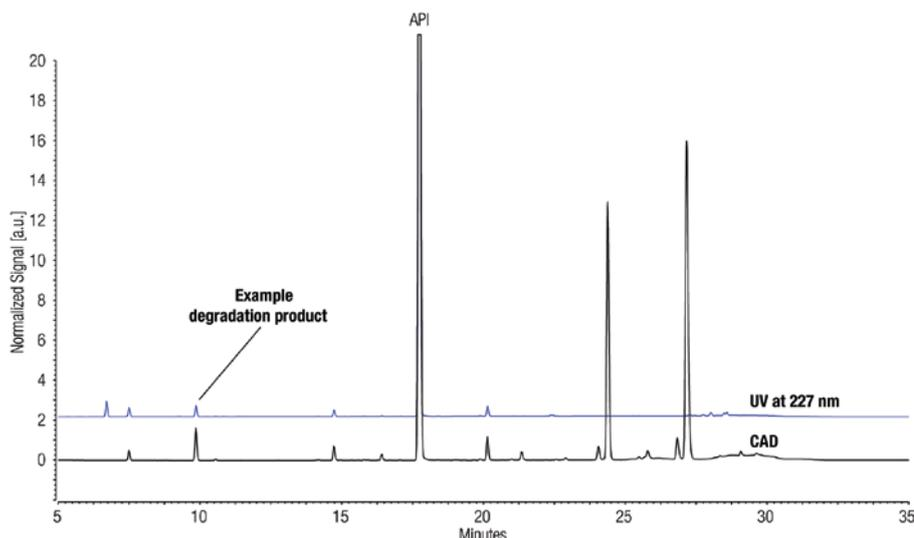
Figure 5: Peak comparison of degradation products between CAD and UV response.
