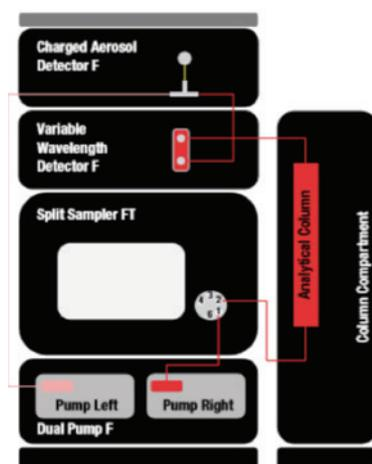
Figure 2: Fluidic scheme of the Vanquish Duo Inverse Gradient Workflow.
