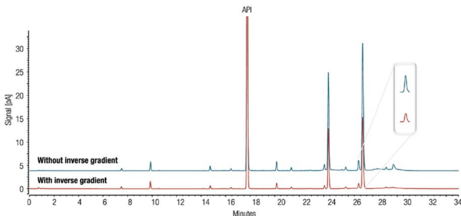
Figure 3: CAD response with and without inverse gradient compensation.
