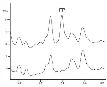
Figure 4: Low-level HPLC detection of FP in dissolution buffer showing baseline interference from trace contaminants in sample diluents arising from concentration of a 2 mL injection volume onto a 50 x 2 mm column. Blue chromatogram (242 nm) = 500 pg/mL spiked dissolution buffer and red chromatogram = blank dissolution media.
