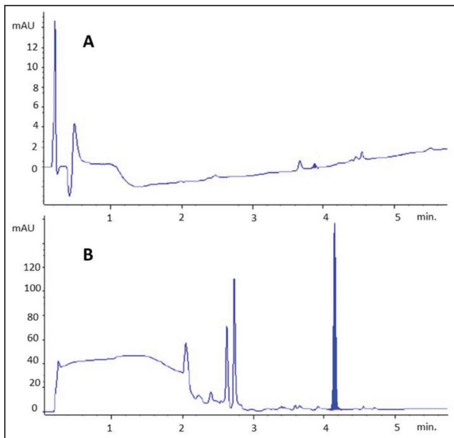
Figure 3: Overlaid chromatograms (242 nm) arising from HPLC analysis of a solution of FP (peak shaded, 100 ng/mL in dissolution media), showing a 400 fold enrichment of FP peak area as a result of increasing the injection volume. A = 5  $\mu$ L injection volume, 500 pg injected through HPLC autosampler; B = 2 mL full-loop manual injection.
