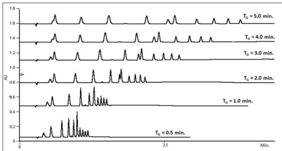
Figure 2: The influence of mobile-phase gradient ramp-rate on peak-shape and resolution of 12 solutes of widely differing polarity [16]. Separations were performed on a 3.0 x 50 mm Luna C18 (1), 3.5  $\mu$ m column with mobile phase flow-rate of 1 mL/min using the Agilent 1100 HPLC system (dwell volume 1.1 mL) and UV detection wavelength of 225 nm. The faster acetonitrile ramp-rates (5-95%) promote focusing and resolution of polar solutes at the expense of narrowing the elution window.
