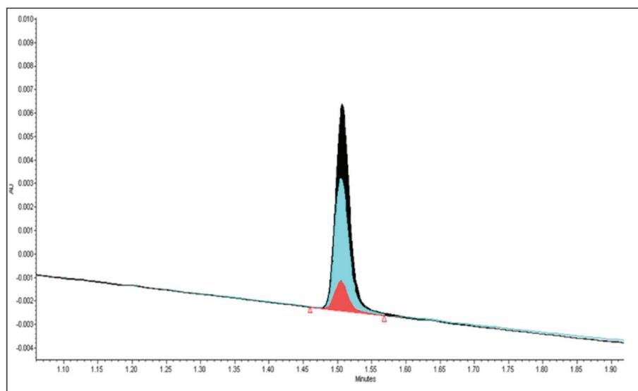
Figure 5: Example chromatograms (242 nm) from optimised high-speed UPLC method with high-sensitivity flow cell showing low-level detection of FP in dissolution samples using 100  $\mu$ L injection with 2 mm I.D. column. Red chromatogram = time-point T1 (10 minutes, 6.1 ng/mL FP), cyan chromatogram = time-point T5 (90 minutes, 18.9 ng/mL FP) and black shaded chromatogram = time-point T10 (900 minutes, 29.1 ng/mL FP).
