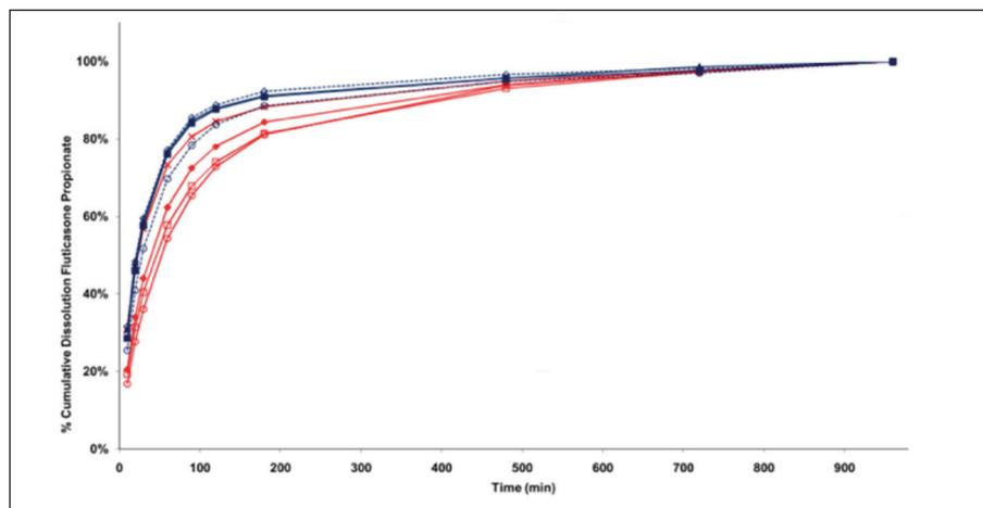
Figure 6: Example cumulative dissolution plots from single-shot FP fine particle doses (100 µg/dose) captured from actuations of eight different developmental dry powder inhaler devices onto filter-disks in NGI device, showing differences in dissolution rates at scales.
