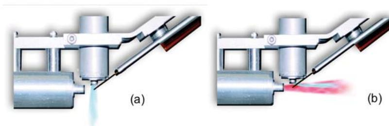
Figure 1: Zoex loop thermal modular. (a) trap with the cold jet; (b) reinject with the hot jet
