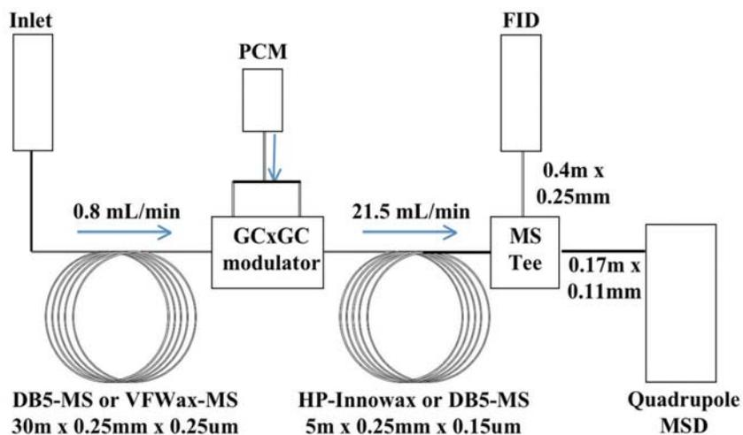
Figure 3: GCxGC-FIDqMSD configuration showing both column sets
