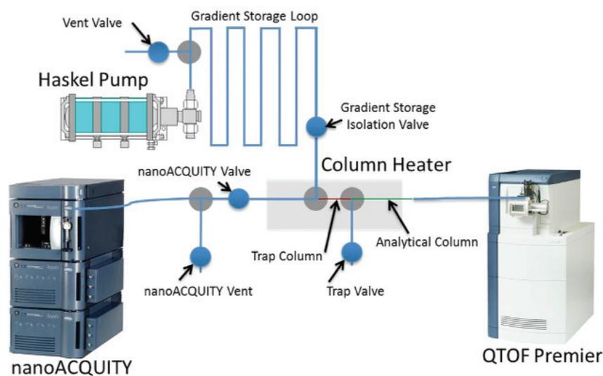
Figure 10: Schematic diagram for the XUPLC add-on to a commercially available UPLC system and associated MS.
