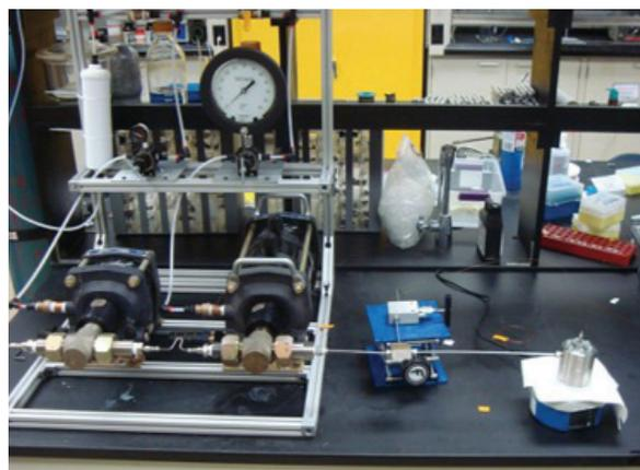
Figure 9: An apparatus used for packing capillaries (typically 75  $\mu$ m id x 1-2 m) for used in XUPLC separations.
